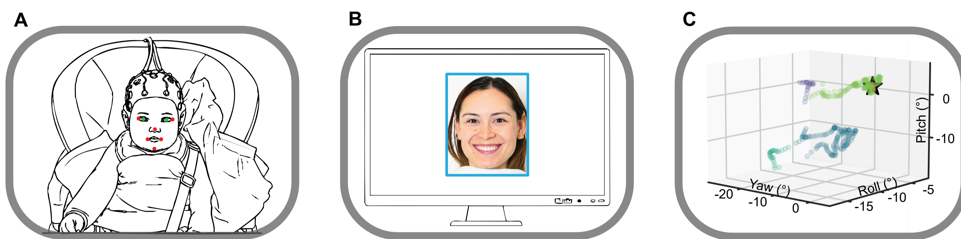
Fig. 2: OCAPI components. A: A CNN (MediaPipe [4]) detects facial landmarks for subsequent head pose and gaze estimation[3]. B: Based on a region of interest and synchronized with event timings, trial onsets are registered. C: A density-based spatial clustering algorithm detects baseline head pose and gaze.
